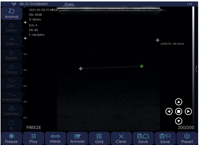
GA (EVD): Embryonic Vesicle Diameter. Calculates the gestation age based on the maximum diameter of the embryonic vesicle.
